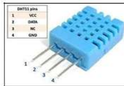
Fig. 2 DT11 Temperature and Humidity Sensor
